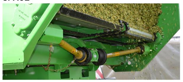
From now on, it is possible to fit the Silo-SPACE silage trailers with a mechanical drive of the moving floor by P.T.O.-shaft and transmission box.
